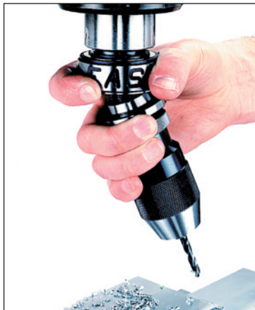
3. Removing drill chuck holder with one hand.
