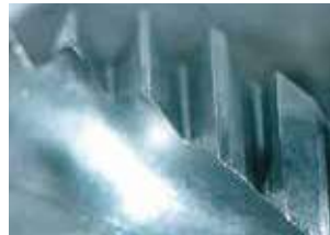
Cutting Edge after Tapping 1,000 Holes
