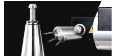
Detector rotation mechanism (0 to 290°, in increments of 1°)
