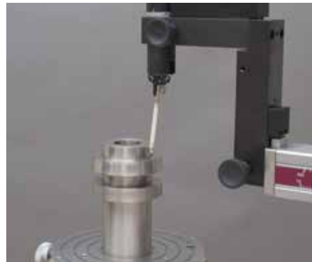
Spiral-mode cylinder measurement
