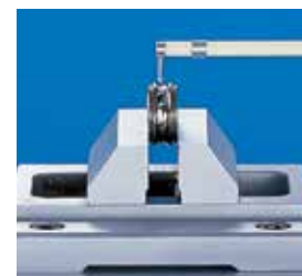
Measuring bearing ring
