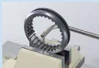
Internal gear teeth
