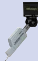
Surftest Probe (surface finish)
