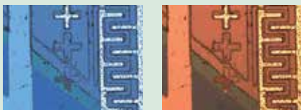
LED illumination | Halogen illumination
